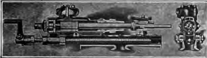
Fig. 16. Longitudinal and Cross Sections through the "Butterfly" Rock Drill, Showing Valve Mechanism and Reservoir Oiler.
